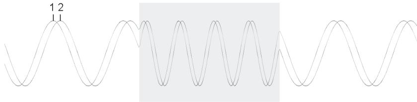
**Fig. 4.21.** Two snapshots of the electric field that propagates across the air and MTM sections at 10 GHz. Trace 1 changes into trace 2 after 10 ps. Clearly, the wave pattern in the air regions has shifted toward the right, while the pattern in the MTM has moved toward the left by half that distance. No scattering occurs at the interfaces by virtue of the impedance match. (*Waveforms generated with the MEFiSto-3D Pro Electromagnetic Simulator by Faustus Scientific Corporation.*)
