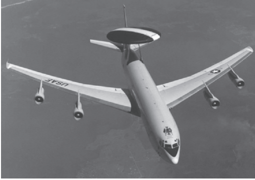
(a) The Boeing 707 showing the radome containing the antenna. (Courtesy of The Boeing Company. Used with permission.)
