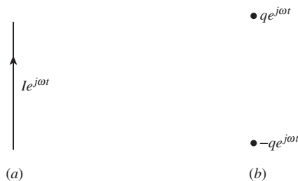
Figure 3-2 Ideal dipole models. (a) Uniform current model. (b) Charge dipole model with I = j\omega q .
