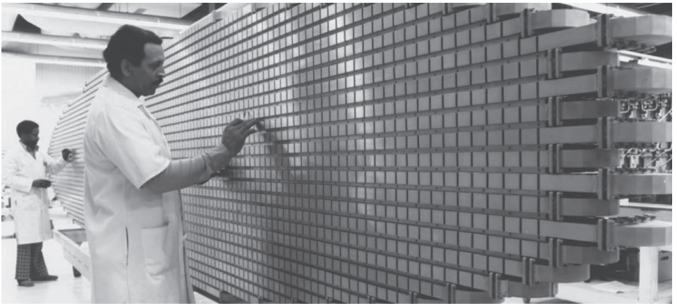
(b) The waveguide slot phased array antenna. (Courtesy of Northrop Grumman Corporation. Used with permission.)
