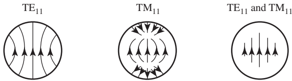
(a) Horn aperture electric field distribution.
