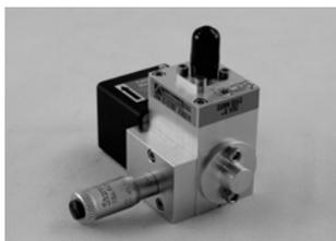
**FIGURE 11.16** A W-band Gunn diode oscillator. The output power is 16 dBm, and the source is mechanically tunable over a frequency range of 4 GHz.
