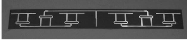
**FIGURE 7.24** Photograph of an eight-way microstrip power divider for an array antenna feed network at 1.26 GHz. The circuit uses six quadrature hybrids in a Bailey configuration for unequal power division ratios (see Problem 7.33).
