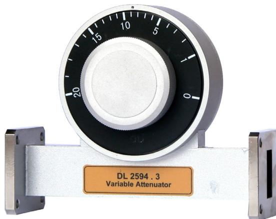
A variable attenuator provides an attenuation by varying the degree of insertion of a matched resistive strip into a waveguide. The variable attenuator is used to control a power level, or to isolate a source from a load. Remarks: the scale is not in dB, the attenuation is only indicative and can be measured by the power sensor.
