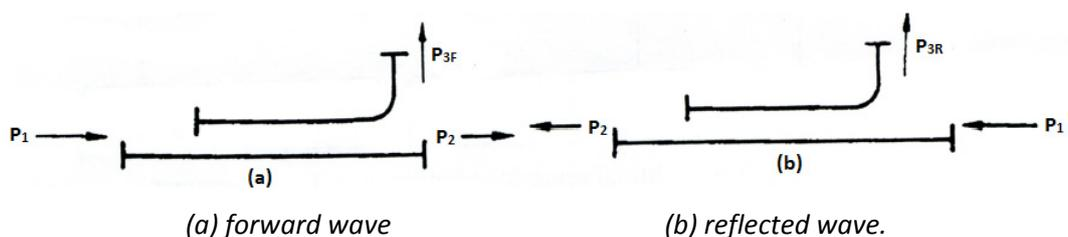
Figure 4.7.2. Sampling direction of a directional coupler.
