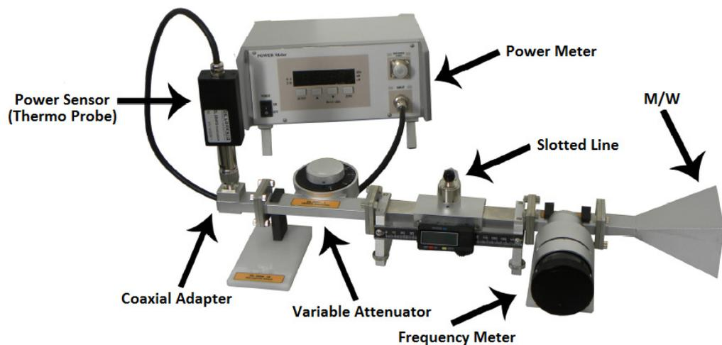
*Figure 2.1. The experimental installation for highlighting the disturbing influences of a metal body introduced into the microwave electromagnetic field propagation environment.*
