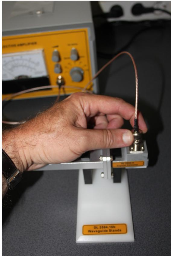
Figure 4.1.20. How to connect the BNC line cord with the Crystal Detector.
