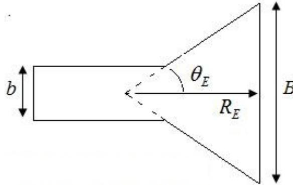
Figure 4.10.6. Cross section of waveguide cut in the E-plane.
