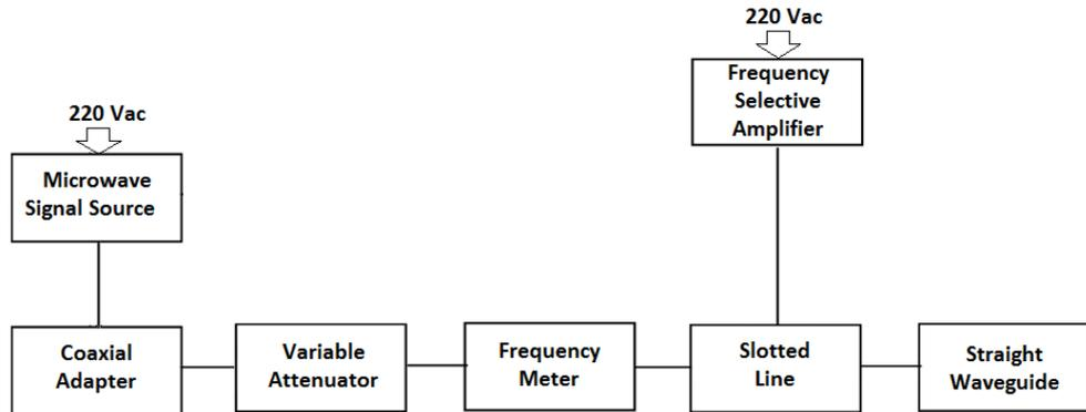
Figure 4.2.2. Equipment setup for measurements of frequency,  $\lambda_g$  and  $\lambda$ .
