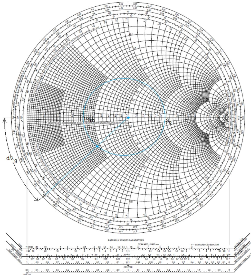
Figure 4.6.4. Finding the load impedance using the Smith chart.
