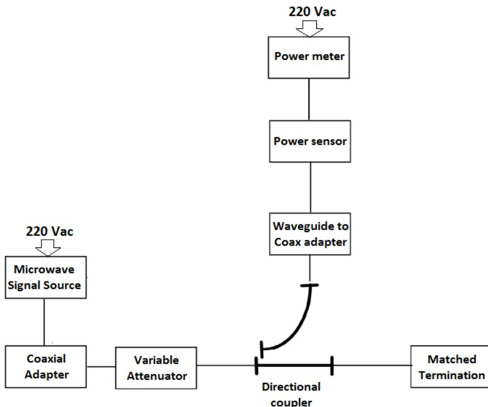
Figure 4.4.5. Setup for power measurement using a directional coupler.
