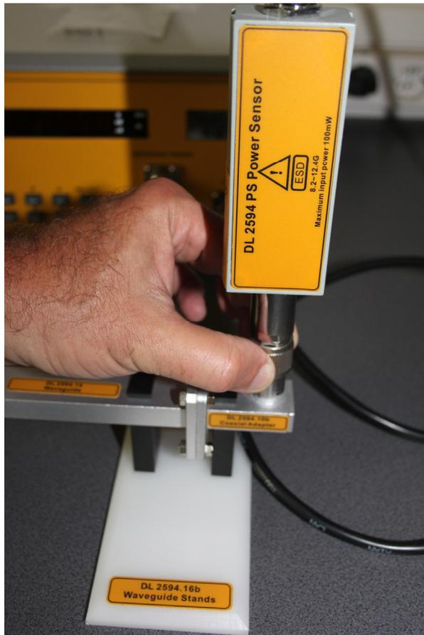
Figure 4.1.8. How to connect the Power Sensor with the Coaxial Adapter.
