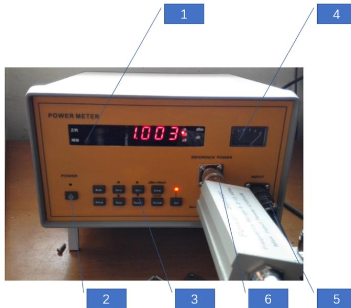
Figure 1. Front panel of power meter
