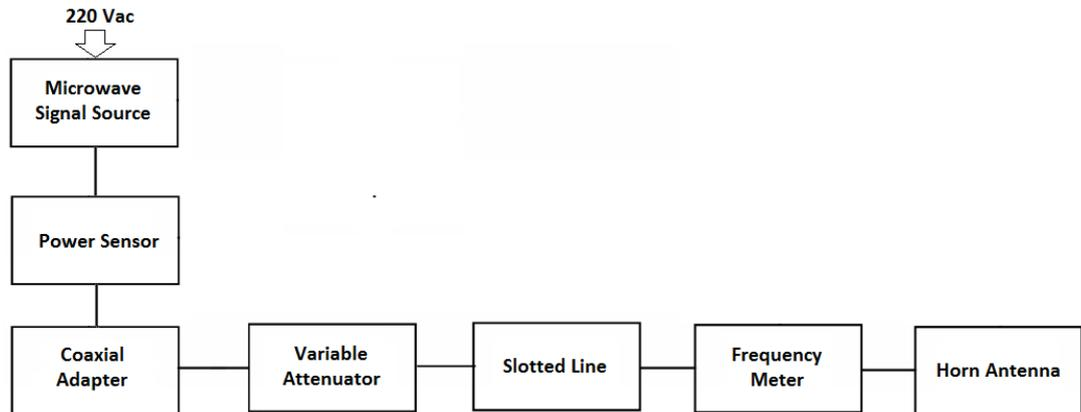
*Figure 1. Experimental module for measuring the influence of the measuring probe on the microwave field propagation characteristics at a given frequency*
