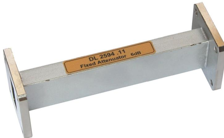
The purpose of the fixed attenuator used in DL 2594N is to provide a fixed attenuation of 6 dB. The attenuation is obtained by the insertion of a thin conducting absorber into a straight portion of a standard waveguide.
