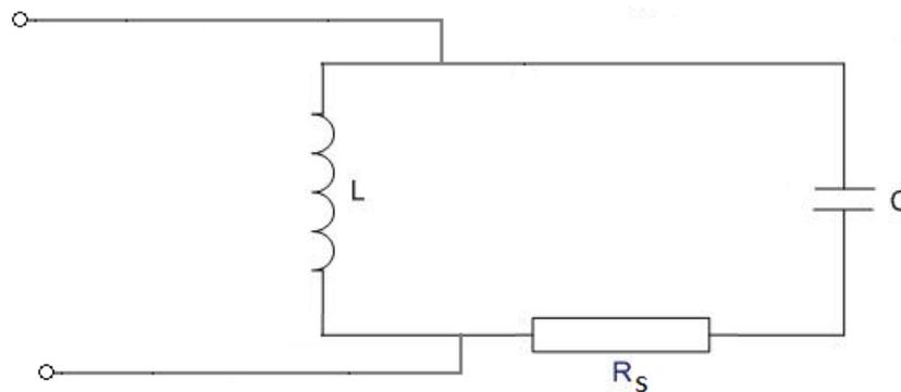
Figure 4.3.1. A resonant circuit.
