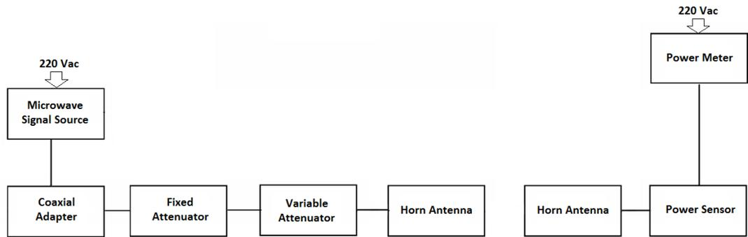
Figure 4.10.8. Setup diagram for measurement of microwave propagation between Horn antennas.
