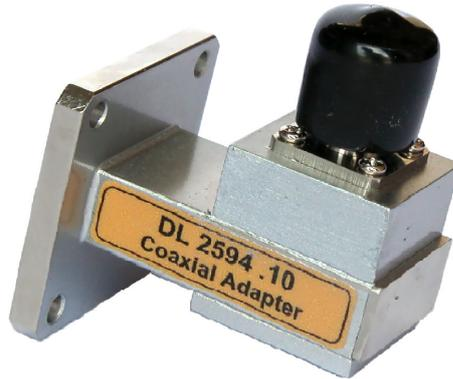
It provides a match between a waveguide and a 50 ohm coaxial line. The power flow can be in either direction. However, the SWR in the adapter should be kept less than 1.2.
