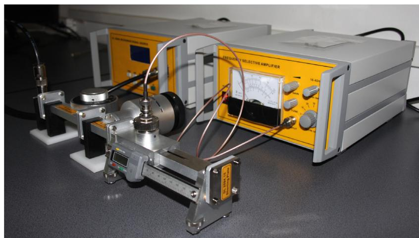
Figure 4.2.6. Real equipment setup for measurements of frequency,  $\lambda_g$  and  $\lambda$  with the Shorting Plate
