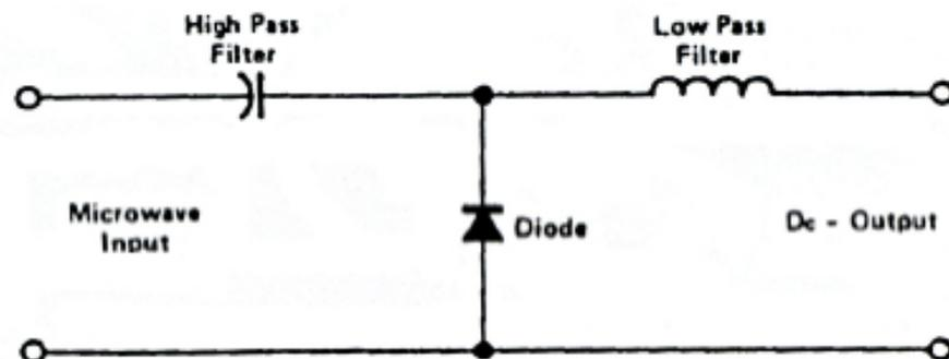
Figure 4.1.1. Typical crystal detector circuit
