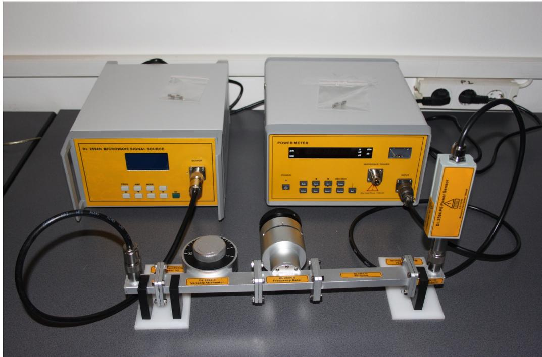
Figure 2.3. DL 2594 PM04 (Power meter) - DL 2594 PM04.1 (Power Sensor)
