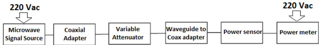
Figure 4.4.10. Setup diagram for measuring the output power of a modulated signal.
