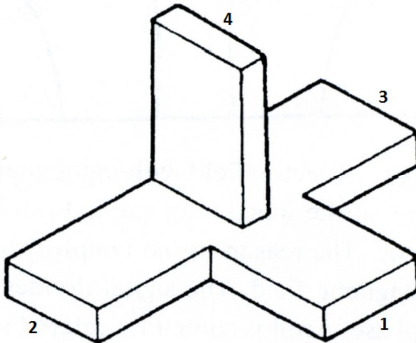
Figure 4.9.1. Waveguide Hybrid-T.
