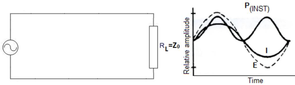
Figure 4.4.1. Instantaneous power appearing at the load resistor.
