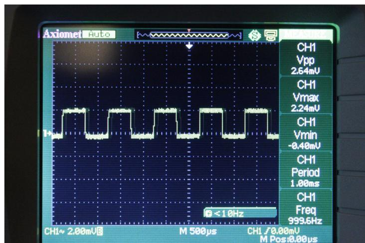
Figure 4.1.8. Square wave modulation and detection on the oscilloscope screen.
