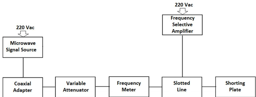
Figure 4.2.5. Equipment setup for measurements of frequency,  $\lambda_g$  and  $\lambda$  with the Shorting Plate
