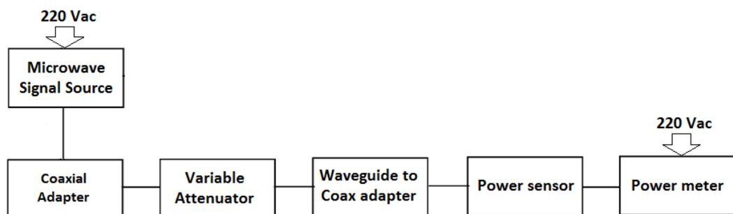
Figure 4.4.3. Direct power measurement setup.
