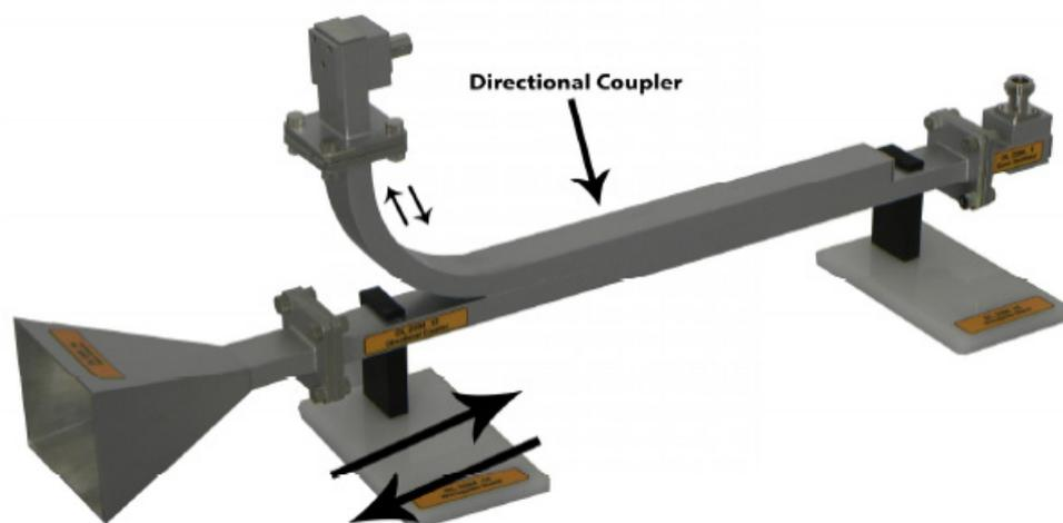
Figure 2.2. The example of using a directional coupler and the arrows indicate the possible wave directions.
