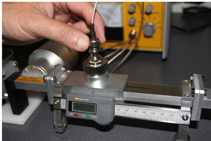
Figure 4.2.4. How to connect the BNC line cord with the Slotted Line.
