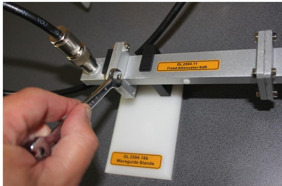
Figure 4.1.14. How to assemble components using screw, nut, and fixed key.
