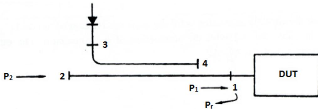
Figure 4.7.3. Return loss measurement.
