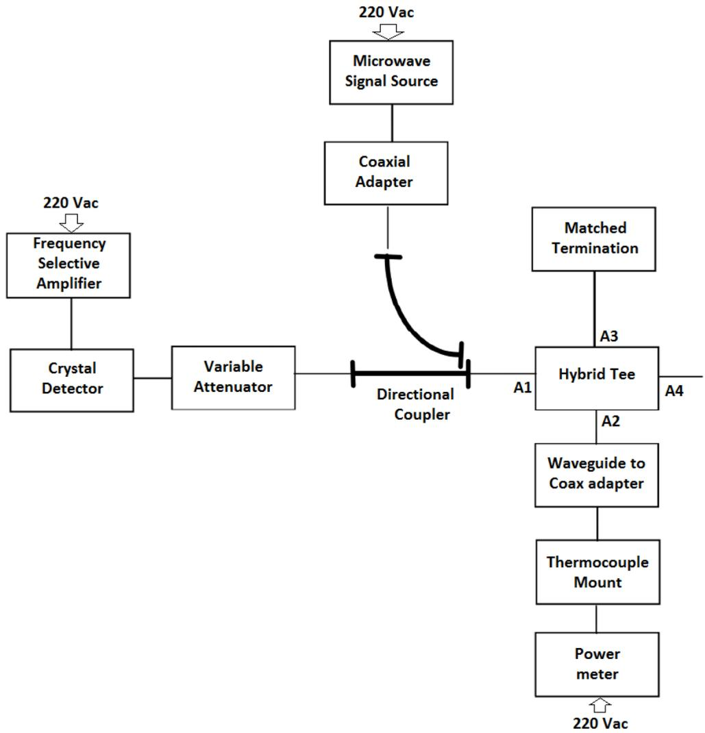
Figure 4.9.12. Return loss measurement setup. The D (5) experiment.
