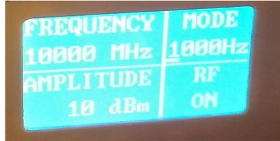
the output mode can be changed by the [MODE] key. When in the amplitude keying output mode, through the [▲ ▼ ◀ ▶] keys you set the required carrier frequency.
