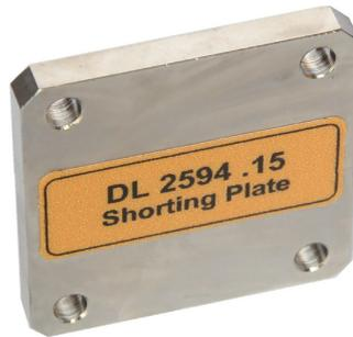
When measuring the wavelength inside of a waveguide, a shorting plate is used to create a short (zero impedance) at the open end of a wave guide.
