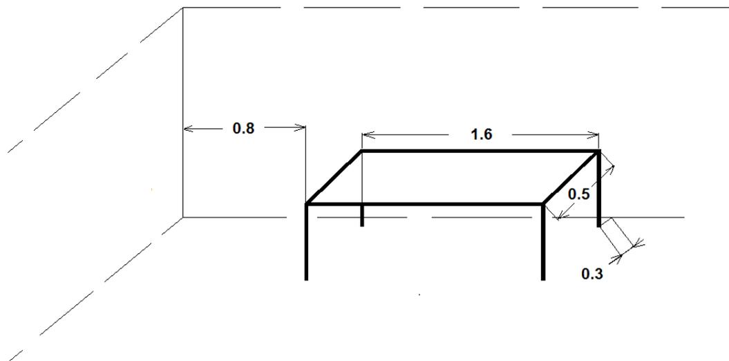
Figure 2.4. The guidance arrangement of the main supports (table) that are used for the DL 2594N Trainer kit.
