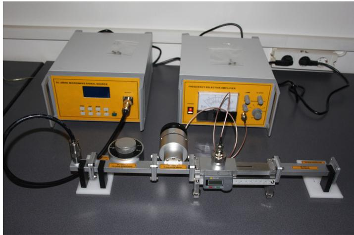
Figure 4.2.3. Real equipment setup for measurements of frequency,  $\lambda_g$  and  $\lambda$ .
