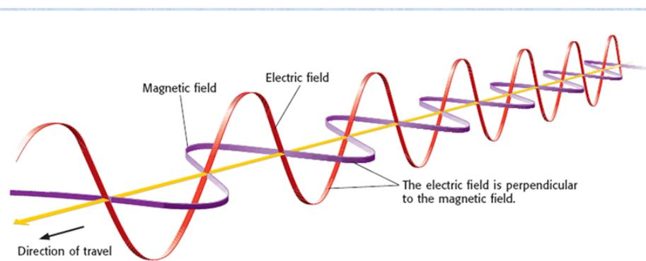
Figure 3.2. The orthogonality property of electromagnetic waves. The pattern.
