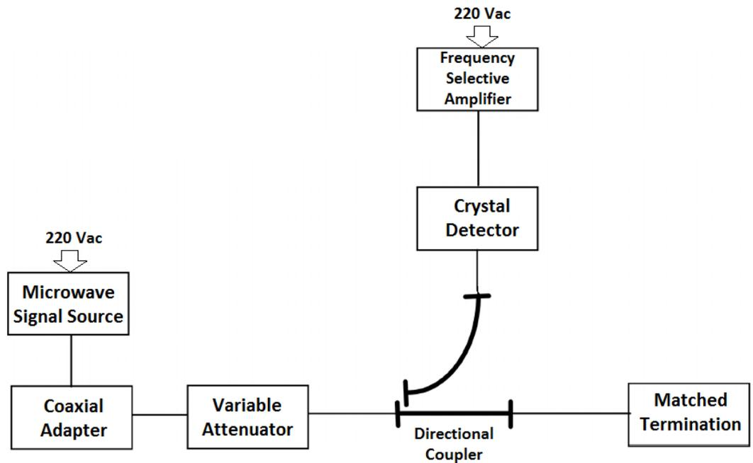
Figure 4.7.6. Setup diagram for coupling factor measurement.
