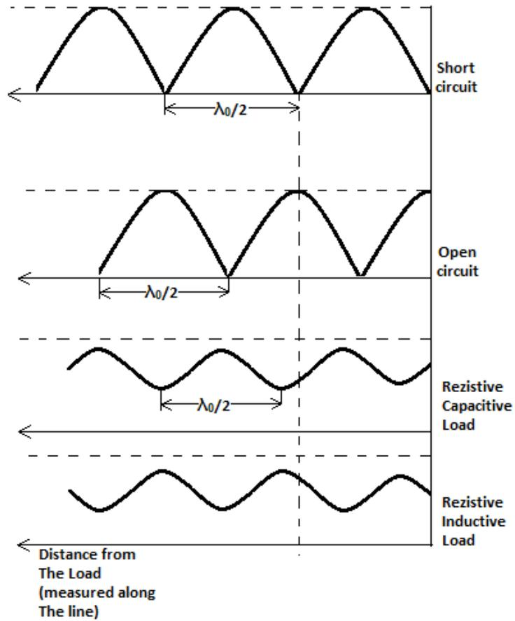
Figure 4.5.1. Standing wave patterns in a lossless line.
