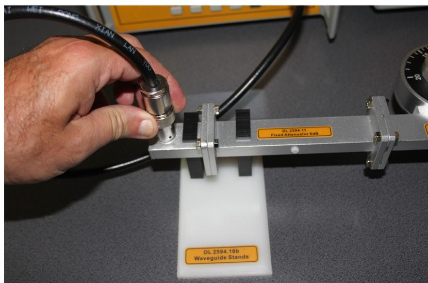
Figure 4.1.15. How to connect the Coaxial Adapter to the line cord with the Microwave Signal Source.
