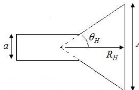
Figure 4.10.5. Cross section of waveguide cut in the H-plane.
