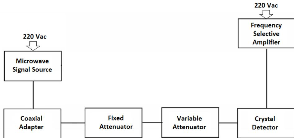
Figure 4.1.12. Setup diagram for measuring the square law characteristics of a crystal detector.
