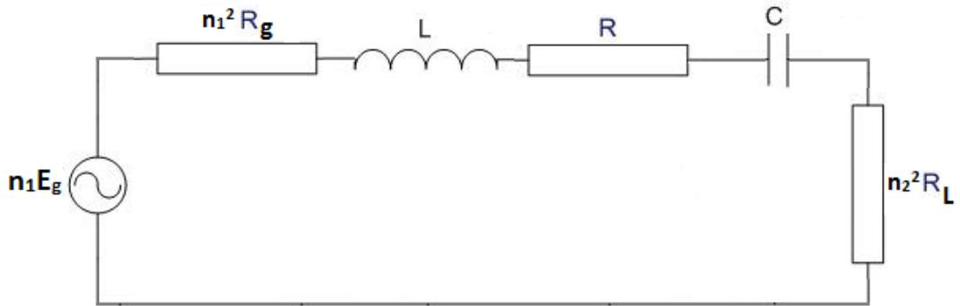
Figure 4.3.3. Equivalent circuit of the cavity portion of Figure 4.3.2(b).
