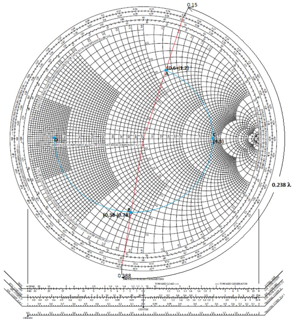
Figure 4.6.2. Solving the example using the Smith chart.
