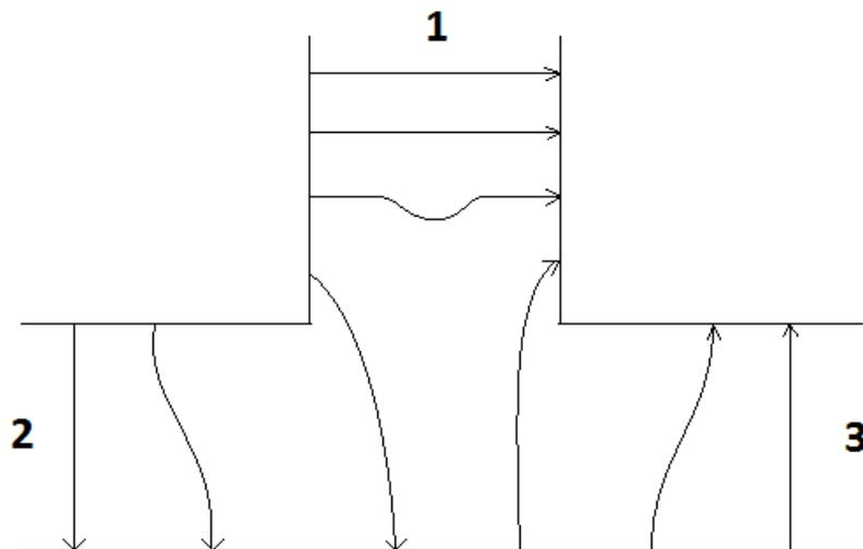
Figure 4.9.3(a). Electric field with input applied at port<sub>1</sub>.
