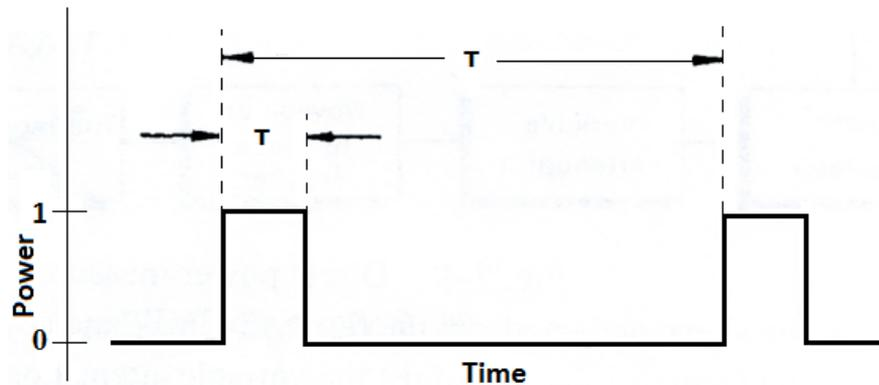
Figure 4.4.2. Peak power of a pulse.
