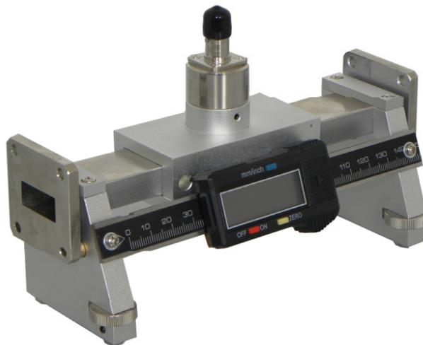
In measuring the standing waves inside a waveguide, a slotted line is used to probe the amplitude and the phase of the standing wave pattern.
