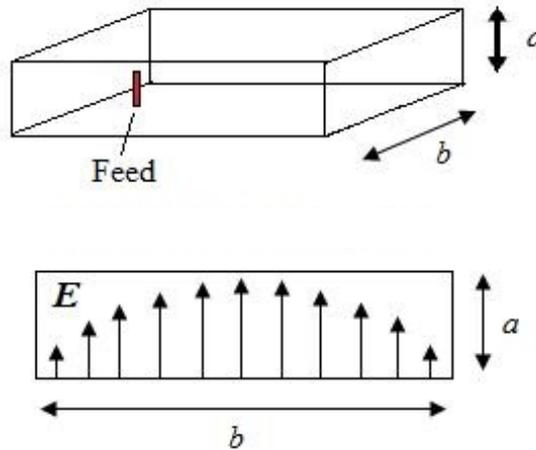
Figure 4.10.4. Waveguide used as a feed to Horn Antennas.
