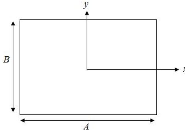
Figure 4.10.7. Coordinate system used, centered on the Horn Antenna opening.
