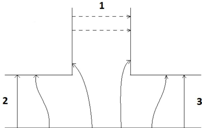
Figure 4.9.3(b). Electric field with input applied at port<sub>4</sub>.
