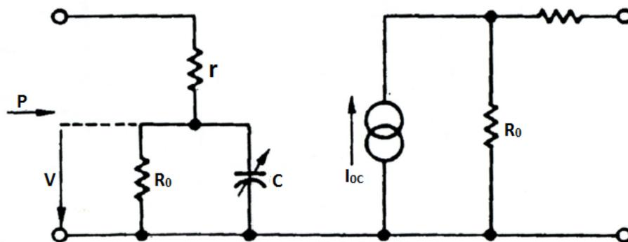
Figure 4.1.3. Equivalent circuit of a detector.
