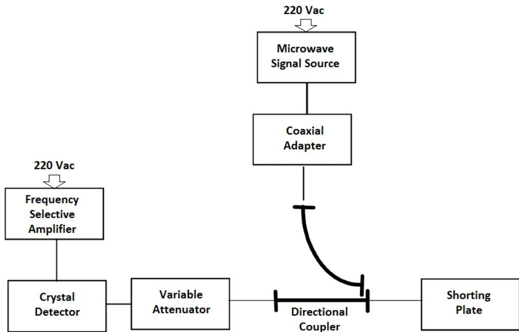
Figure 4.9.9. Initial setup for return loss measurement.
