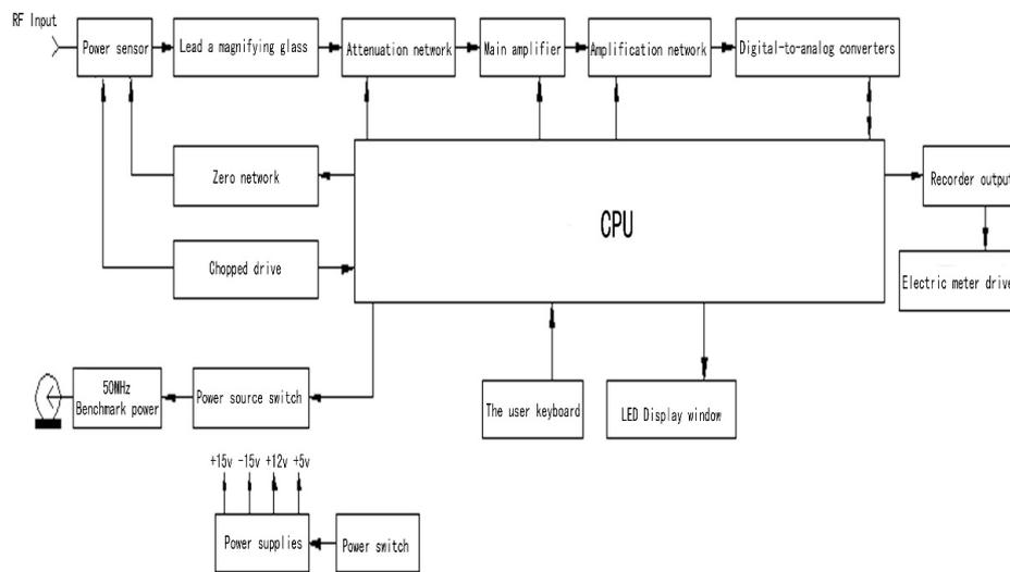
Figure 2. Power Meter Principle Block Diagram
