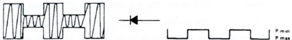
Figure 4.1.7. Square wave modulation and detection.
