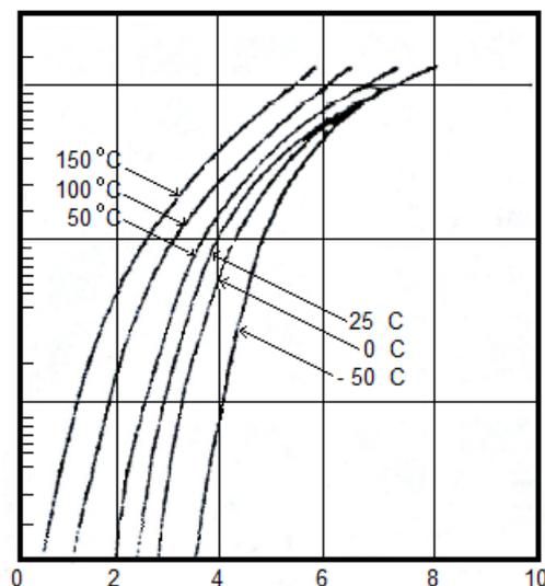
Figure 4.2. The V-I characteristics of a crystal diode. Forward Voltage
