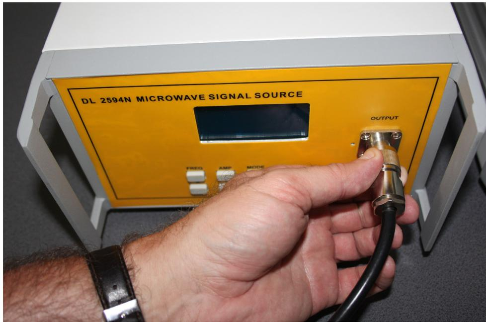
*Figure 4.1.16. How to connect the line cord with the Microwave Signal Source.*
