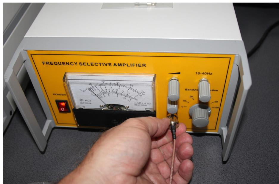
Figure 4.1.19. How to connect the BNC line cord with the SWR Meter.
