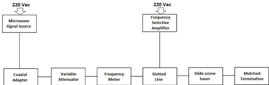
Figure 4.6.5. Setup diagram of impedance measurement.
