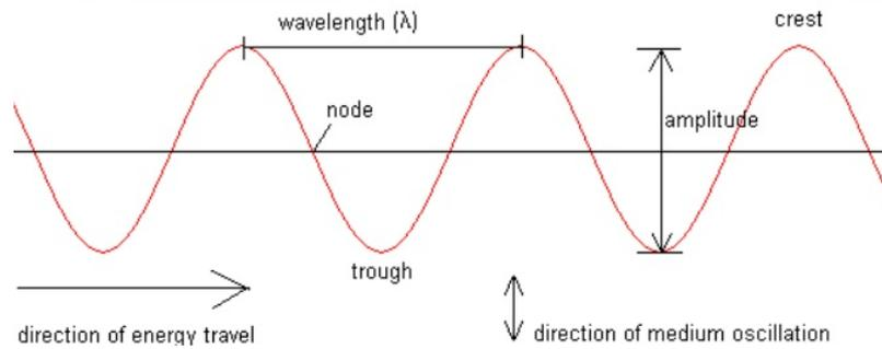
Figure 3.1. Waves main parameters
