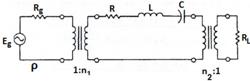
Figure 4.3.2(b) An equivalent circuit of Fig. 4.3.2(a).
