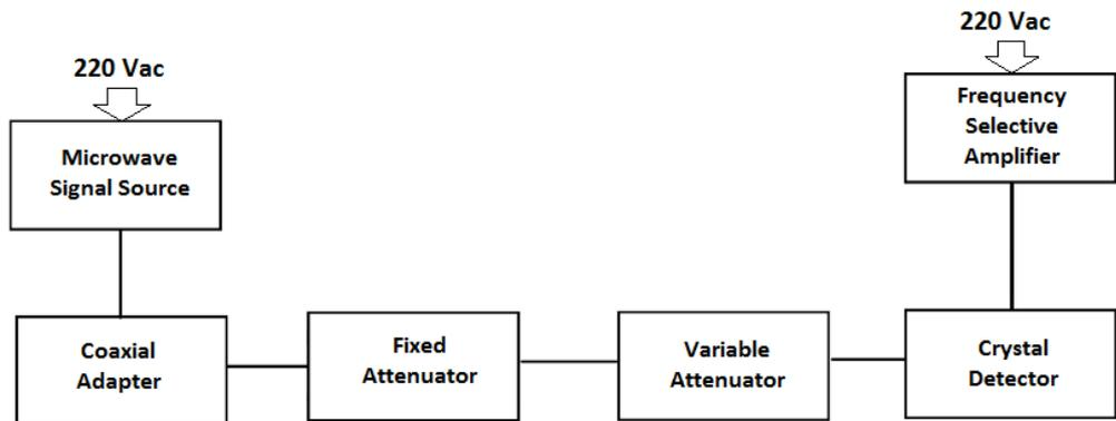
Figure 4.9.4. Initial setup diagram.
