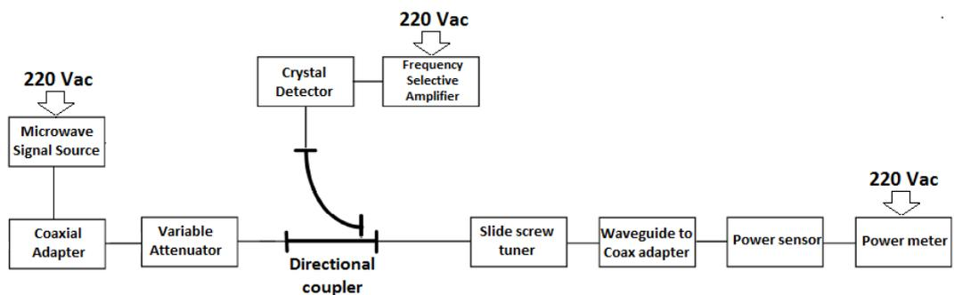
Figure 4.4.9. Setup for measurement of conjugate and  $Z_0$  power.
