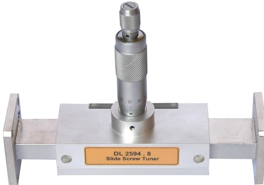
The primary use of the slide screw tuner is to match loads, detectors, or antennas to the characteristic impedance of the waveguide. The mechanical structure of a slide screw tuner consists of a probe mounted on a carriage which slides along a narrow and long slot on the feeding waveguide. When the adjusting micrometer is turned, the depth of the probe varies. The combination of the depth and the position of the probe causes a reflection in the waveguide at a specific amplitude and phase.
