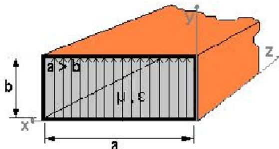
Figure 4.2.1. Rectangular waveguide in a rectangular coordinate system.
