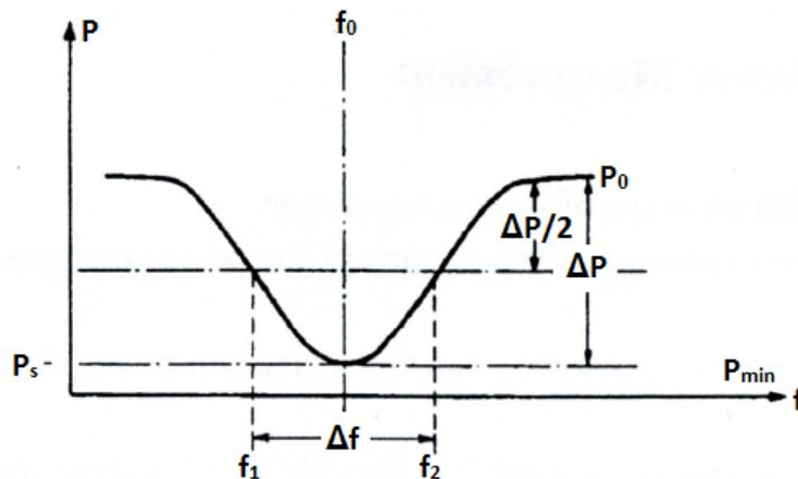
Figure 4.3.6. The resonant curve of a resonant cavity.
