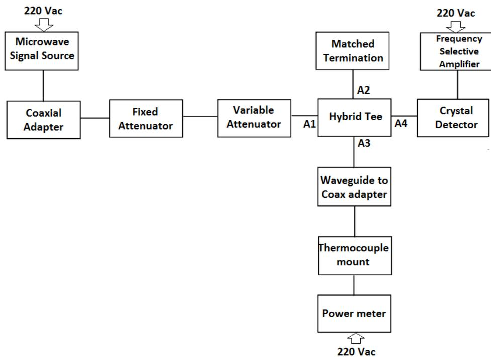
*Figure 4.9.6. Setup diagram for measurement of decoupling between H Arm and E Arm.*
