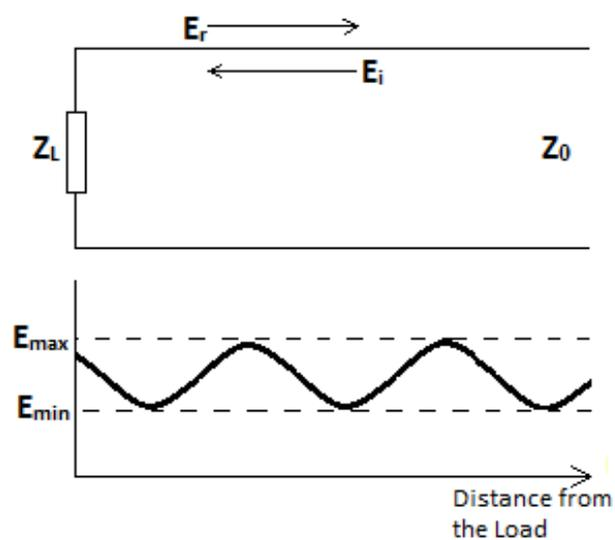
Figure 4.5.2. A voltage standing waveform.
