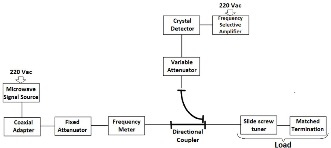
Figure 4.7.10. Setup diagram for return loss measurement.
