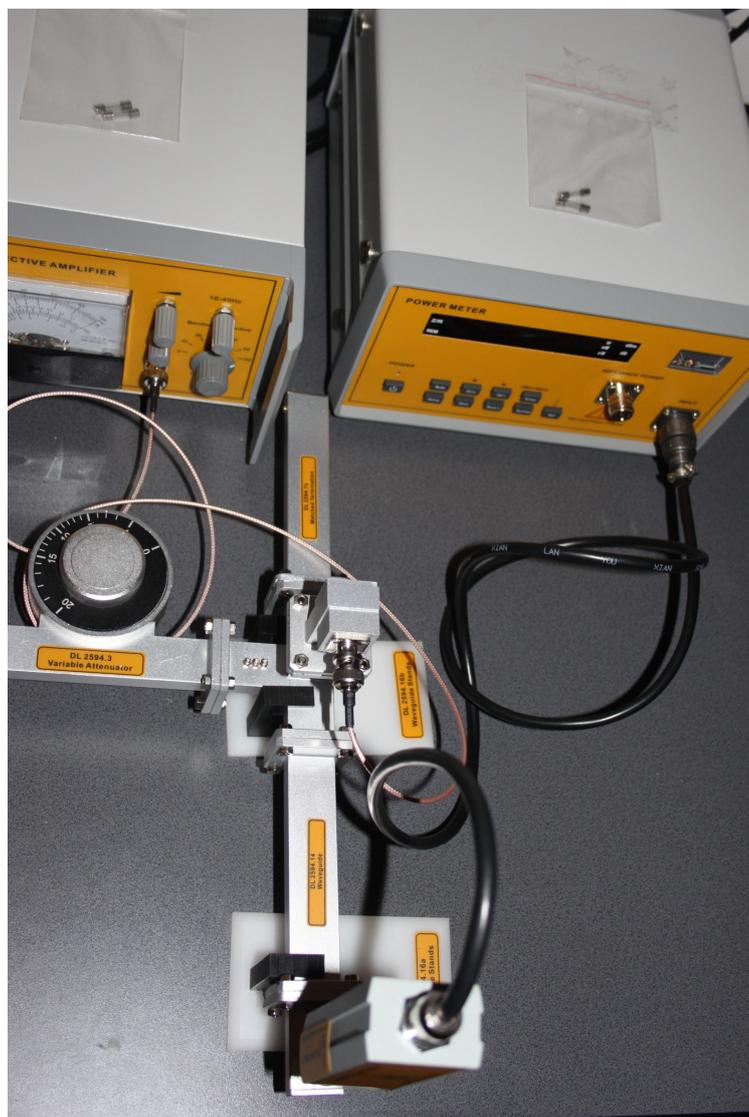
Figure 4.9.8. Detailed picture on connecting components to Hybrid-Tee.
