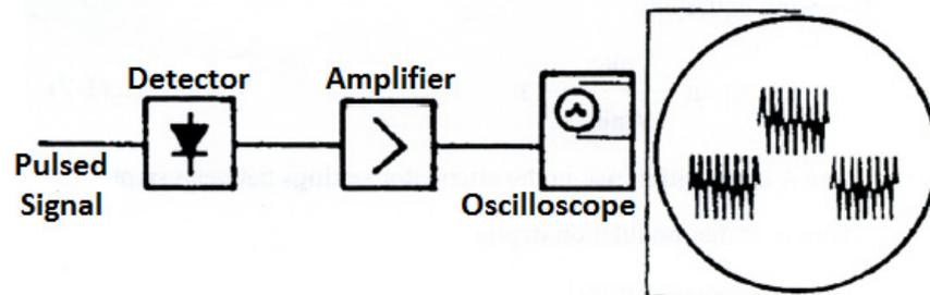
Figure 4.1.4. The TSS of a diode.
