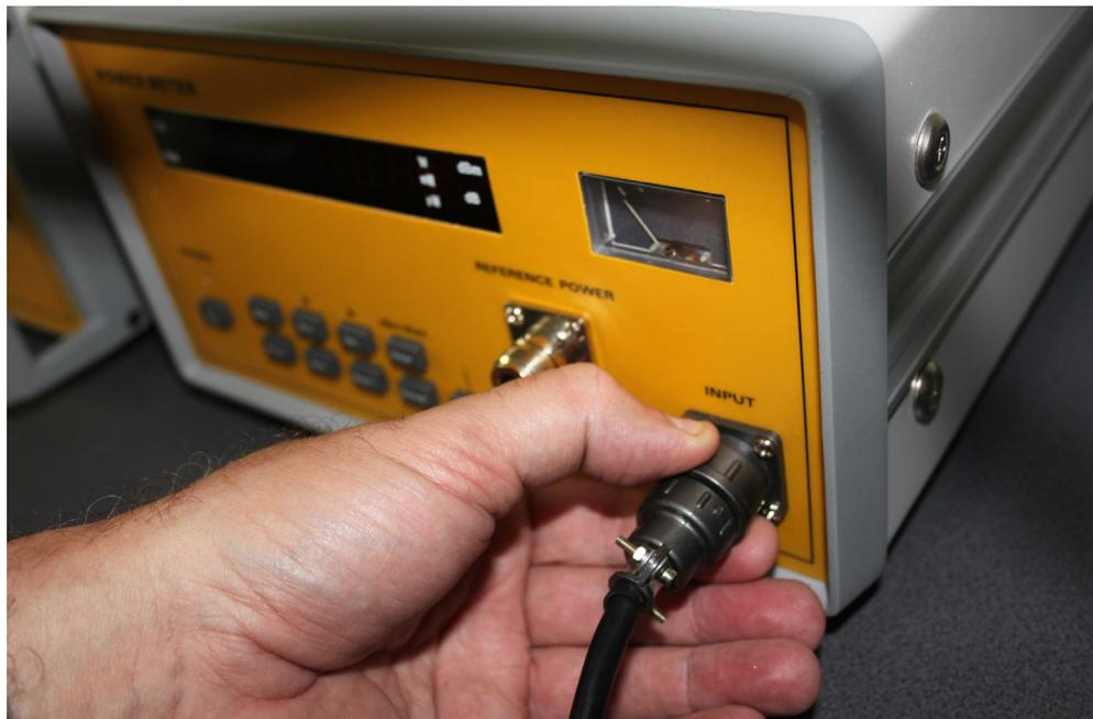
*Figure 4.1.17. How to connect the line cord with the Power Meter.*
