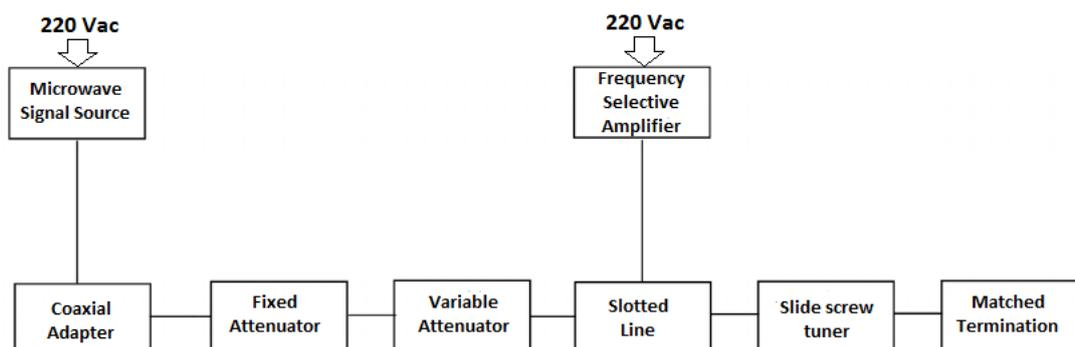
Figure 4.5.3. Setup diagram for SWR measurement.
