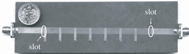
**Fig. 5.53.** Prototype of a 7-cell microstrip CRLH TL (Section 3.3.2) open-ended resonator. Coupling is achieved via two weakly capacitive slots of width  $200\ \mu\text{m}$  on the input/output microstrip traces at the edges of the structure. The substrate used is Duroid 6510 with permittivity 2.2 and thickness 1.57 mm.
