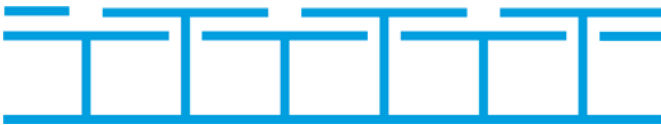
Figure 11.9 Thin high-impedance surface with a low resonance frequency can be built by using greater capacitive loading, such as overlapping plates, as shown in this three-layer structure. For a given resonance frequency, thinner structures have smaller fractional bandwidth.
