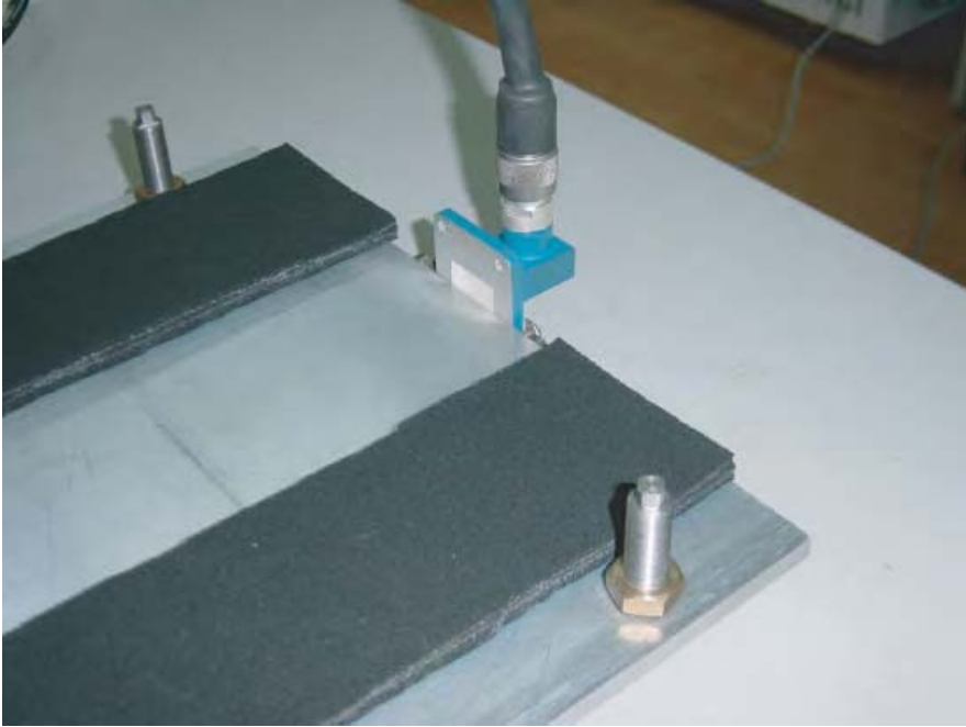
Figure 4.3 Picture of waveguide coupler being fed into PPW (in which top plate has been removed).
