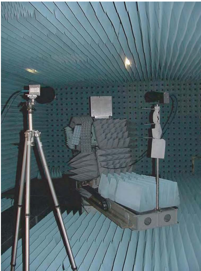
Figure 9.5 Photo of setup for measuring EBG reflection phase as function of frequency for different angles of incidence using feedhorns to launch and receive radiation in anechoic chamber.
