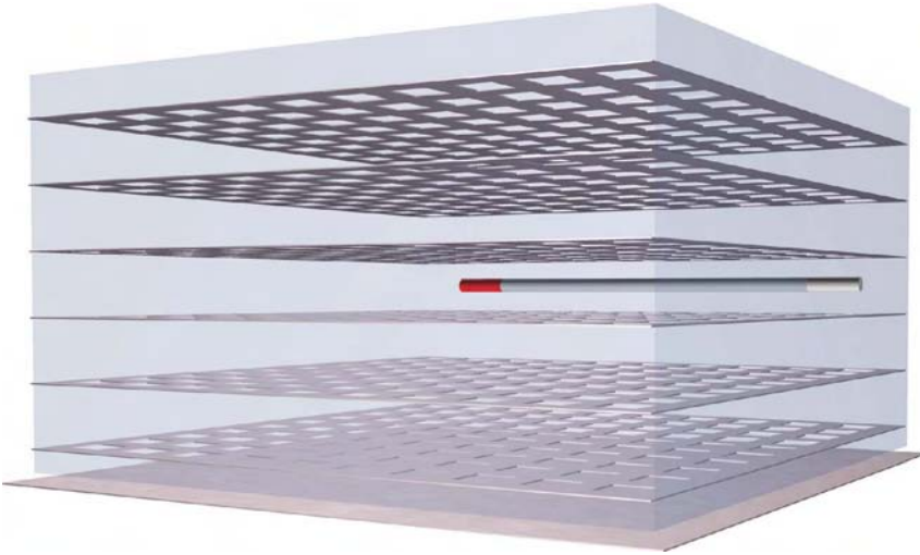
Figure 10.11 Schematic representation of antenna. The six copper grids are separated by foam. The rod in the middle represents the coaxial cable ended with the monopole (in red). The bottom plane is the ground plane.
