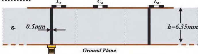
Figure 5.21 Diagram of MTM ring antenna at 1.5 GHz. The loading capacitance and inductance required to feed the vias in phase are C_0 = 3.70 pF and L_0 = 71.08 nH.
