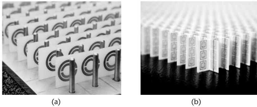
Figure 8.1 (a) First experimental demonstration of LHM [5] and (b) a 2-D isotropic LHM [6].
