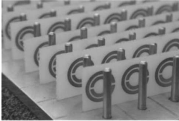
Figure 1.8 Realization of DNG material at microwave frequencies [4].
