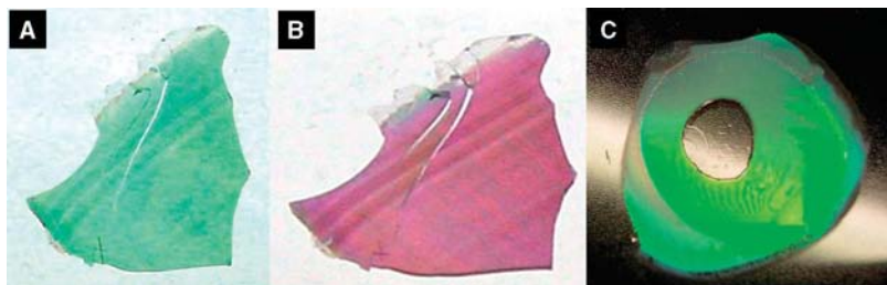
Figure 3.10 Ormocer inverse opal (A) free standing film – top view, (B) free standing film – tilted viewing angle, (C) replica on a glass substrate (2 cm×2 cm) [46].
