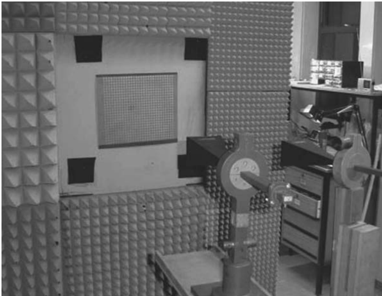
FIGURE 31.9 Experimental setup for testing the AMC performance.
