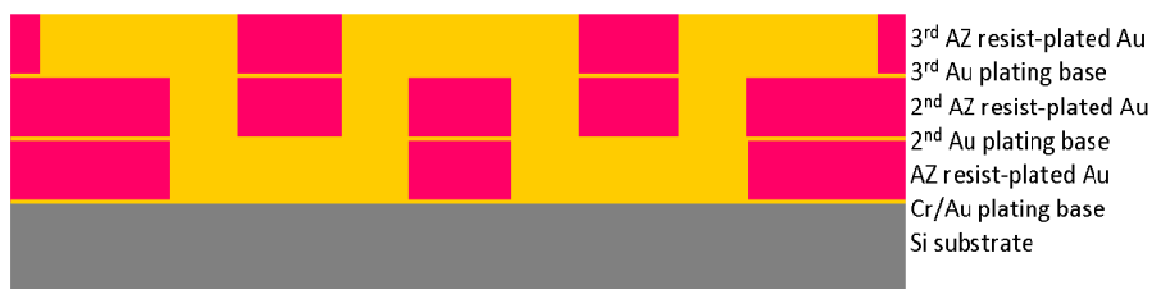
Fig. 6: Fabrication of the meta-foil by means of multilayer lithography with precise alignment and gold electroplating with accurate thickness control.
