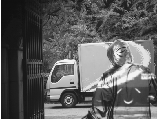
Figure 10.5. Adaptive camouflage. (From the Tachi Laboratory, Keio University and The University of Tokyo, courtesy of Professor Susumu Tachi.)
