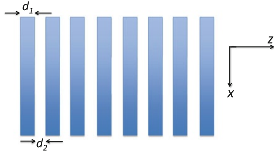
Fig. 10.14 Schematic of a composite material consisting of a periodic arrangement of two different materials with widths of d_1 and d_2 , respectively
