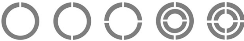
Fig. 1.4 Some split ring resonators designed by Aydin et al. [15] (Reproduced with permission from Fig. 11 of [15])
