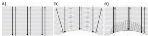
Figure 7.15. Two-dimensional numerical simulations for the diffraction of an SPP: a) on a flat mirror; b) on a curved mirror; c) on the curved mirror in presence of the metamaterial (cylindrical dielectric pillars of TiO_2 ) for a wavelength of 800 nm
