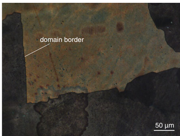
Fig. 3.5 Domain morphology of gyroids obtained by drying-annealing. The image was obtained by optical microscopy under linear polarized light after metal replication. As discussed in the next chapter, the metal gyroids show a strong linear dichroism that enables the inspection of the domain size
