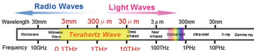
Fig. 3.15 THz regime of the EM wave lies between electronic (microwave) and photonic (IT) frequency, and extends from 100 GHz to 10 THz (Origin: http://www.fujitsu.com/global/about/resources/news/press-releases/2011/0912-01.html )
