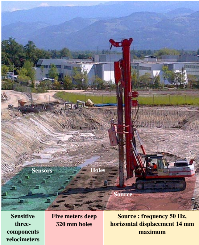
Fig. 7.13. Photo of the experimental setup of the seismic field test in Grenoble (Summer 2012), where the region highlighted in green is protected from surface seismic waves generated by a source (crane with rotating head at 50 Hz) thanks to the array of boreholes (region highlighted in blue). Boxes on the soil are velocimeters.
