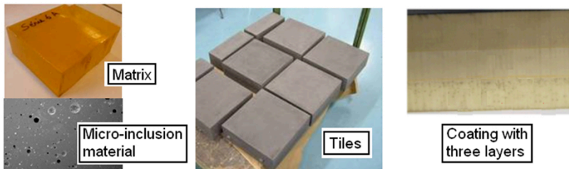
Figure 9.13. Acoustic coating technology using micro-inclusion materials
